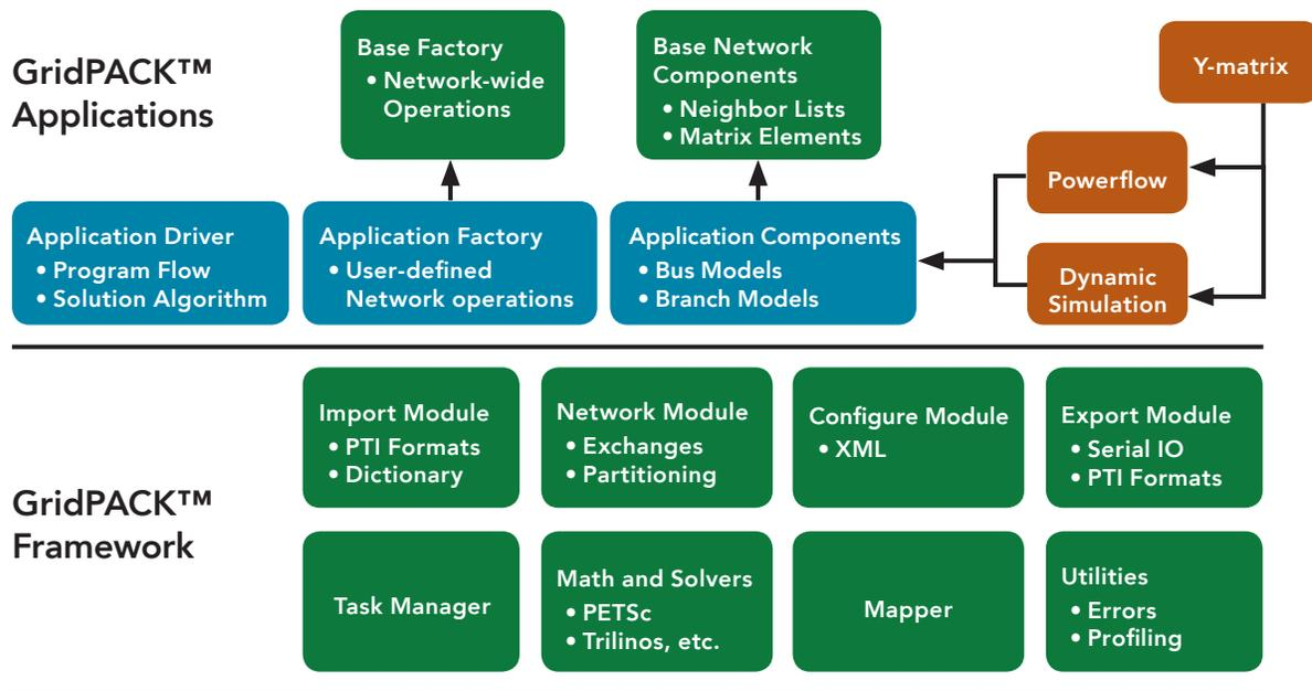
*Schematic diagram of the GridPACK™ Software Stack*
