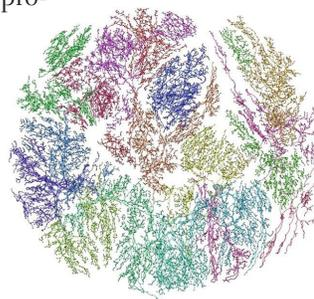
This representation of the Western Electricity Coordinating Council network illustrates how GridPACK™ partitions the network onto 16 processors. The partitioning divides the network into separate pieces that can be worked on concurrently using multiple processors to improve computational performance.
