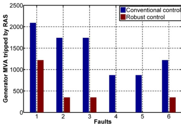
Minimum machine capacity to be tripped by remedial action schemes to ensure system stability
