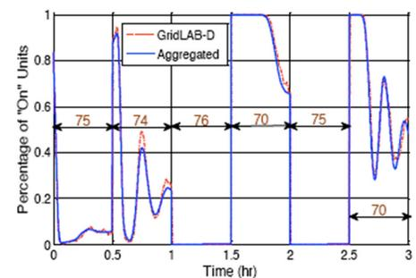
*Validation of Aggregated HVAC Model with Detailed Model*
